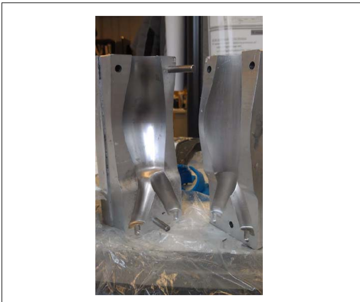
Figure 20: AAA mold aluminum blocks milled using a CNC machine. Dowel pins are used to ensure the two halves of the aluminum block are perfectly aligned.
